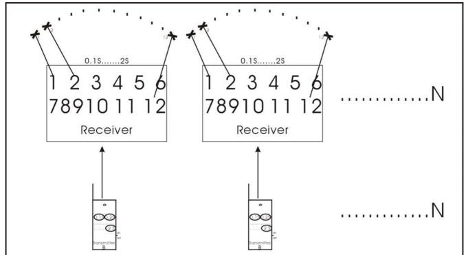
3, Cancel all the frequencies previously programmed into the receiver first. Then different transmitter B (from the sequence of 0.1s to 2second) will be programmed to different receivers separately.
