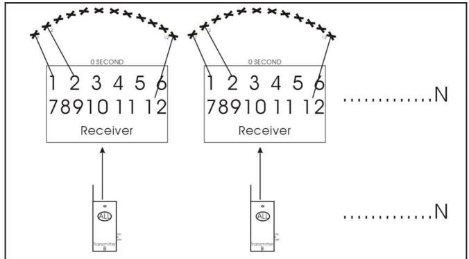
5, Cancel all the frequencies previously programmed into the receiver first. Then different transmitter B will be programmed to different receivers separately. EFFECT: When you press the button(ALL) of the transmitter B, then all the channels of the receiver which is belong to this transmitter will be fired all together(0second). See photos, please.
