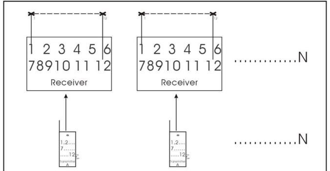
1, Cancel all the frequencies previously programmed into the receiver first. Then different transmitter A will be programmed to different receivers separately. EFFECT: when you press the button of transmitter from 1 though 12 and will only fire one channel of the receiver which is belong to this transmitter at a time. See photos, please.
