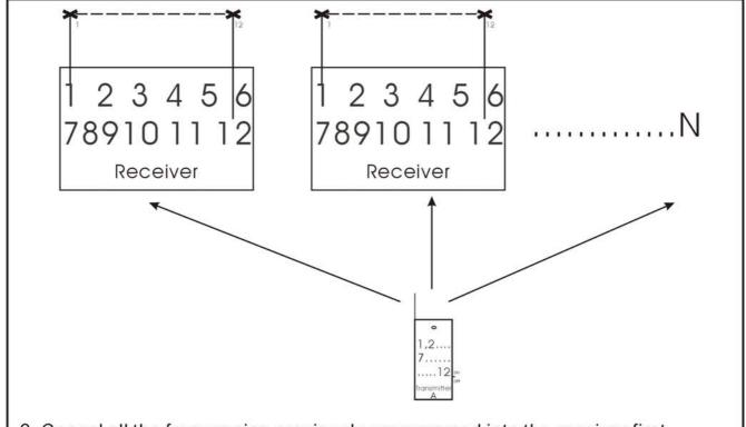
2, Cancel all the frequencies previously programmed into the receiver first. Then get one transmitter A to be programmed to many(N) receivers. EFFECT: when you press the button from 1 though 12 and will only fire one channel of each receivers at a time. See photos, please.
