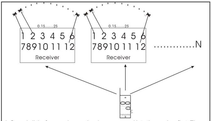
4, Cancel all the frequencies previously programmed into the receiver first. Then get one transmitter B (from the sequence of 0.1s to 2second) to be programmed to many(N) receivers.
